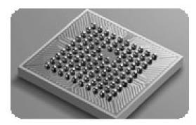
Figure 3. IC in flip chip technology
