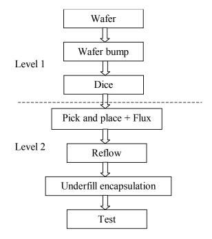
Figure 4. The flip chip process flow
