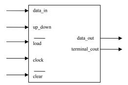
Figure 1. A 4-bit loadable up/down counter
