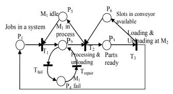
Fig.7. FIPN model for the production line
